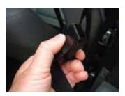
Lift the tab on the adjustment buckle to change the length of the strap if needed to make it taught. Relock the tab to secure the strap.
