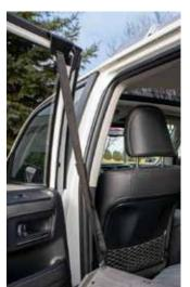
The Side Entry Support Strap will now be secured in place and supporting the corner of the ramp, preventing it from tipping.
