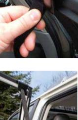
The Side Entry Support Strap will now be secured in place and supporting the corner of the ramp, preventing it from tipping.
